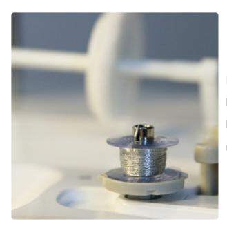
Now it is time to sew the first lace piece. Since both sides of the lace petals will be seen, wind a bobbin with the same thread as used in the top needle.
