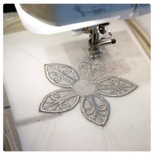
Then hoop a piece of heavy water-soluble stabilizer tightly, and load the first lace piece (labeled with a "b"). Embroider the design.
