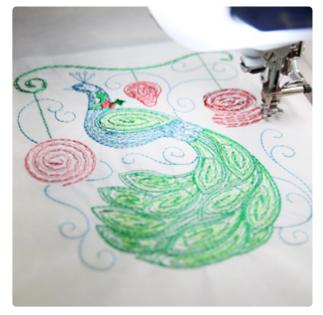
Attach the hoop back onto the machine and continue with the design. After each stop, remove the hoop, trim any loose bobbin threads, change the bobbin to the next color, and match the top thread to the bobbin thread.
