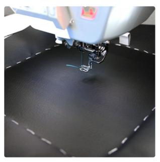
Another option for faux leather is to float the fabric on the hoop. Floating the fabric is when the stabilizer is hooped firmly by itself. The fabric is then hand sewn onto the stabilizer. This way the hoop never pinches the fabric, and there is no chance for hoop burn.
