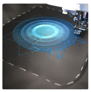
Attach the hoop onto the machine and load the embroidery file. Use a 75/11 sharp sewing needle. This type of needle has a finer point and will make smaller perforations in the stabilizer and fabric. Follow the color change sheet and embroider the design.
