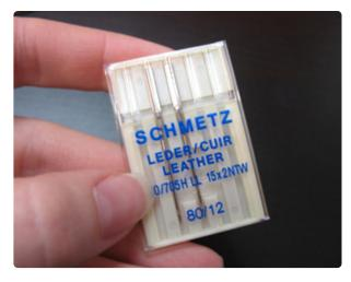
Needles! This is an important one. A size 80/12 leather needle is a good choice when embroidering onto leather. This kind of needle has a wedged point that reduces the size of the hole or perforation made in the leather.
