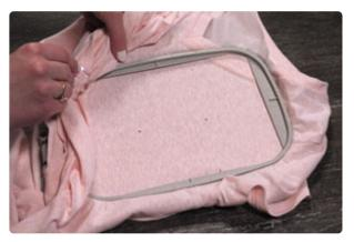
Hoop both fabric and stabilizer together, taut in the hoop to prevent shifting and gapping while your design stitches.
