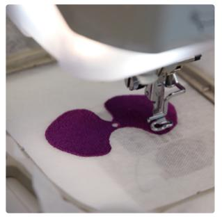
Load the embroidery design onto the machine, and place the first thread color and matching bobbin into the machine. Then begin to embroider the design.
