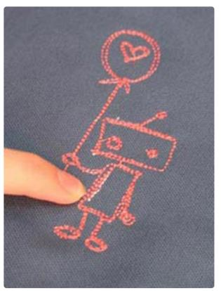
Once you're done sewing, check to make sure your design looks ok. My little robot has some tension issues. Perhaps he didn't get enough hugs as a wee bot. Do you see that white thread on the top? That's the bobbin thread not behaving. To fix this, adjust the tension on your machine, shown below. And if you're really lazy (or some would say efficient), use a colored marker to fill in the white bits.
