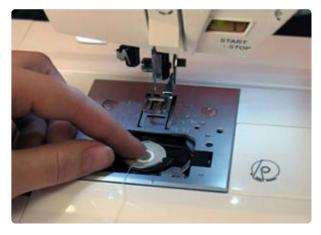
Open up the shiny cover that slides over the bobbin case and insert a bobbin. Your machine might have come with bobbins, but if not you can wind one (refer to that manual again!).
