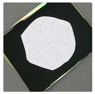
Spray the back side of the printed paper dieline with temporary spray adhesive and place it on the back side of the backing fabric. Placing the paper dieline on the back of the fabric instead of directly on the Mylar will prevent the adhesive from being left on the Mylar.
