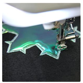
Then place the hoop back onto the machine and embroider the tackdown for the applique piece.
