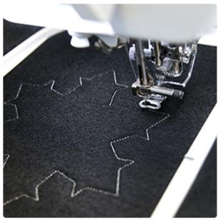
Attach the hoop onto the machine, and load the embroidery file (not the dieline files).
