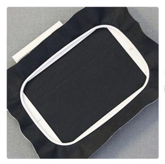
Hoop the fabric and stabilizer firmly. Make sure it is nice and tight with no wrinkles.
