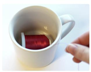
Here's a trick some embroiderers swear by, especially for metallic thread: place your spool of thread in a coffee cup, set it next to your machine (or on the floor nearby, for even more distance), and thread the machine as usual. This gives the thread more space to unwind, preventing kinks that could cause the thread to break. Make sure the thread can't get caught anywhere between the cup and the machine.
