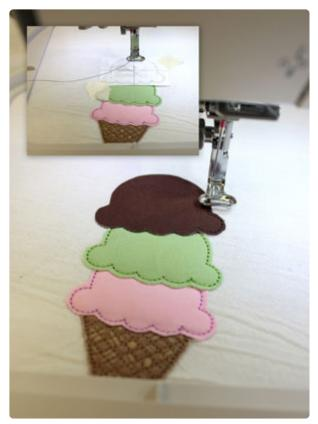
Place your hooped design under your machine, and make sure your needle is under the crosshairs, or your trace shows that your design is placed correctly.
