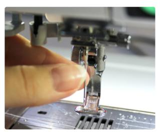
Any burrs on the needle could also contribute to thread breaks, so use a fresh needle to make sure it's in good condition.
