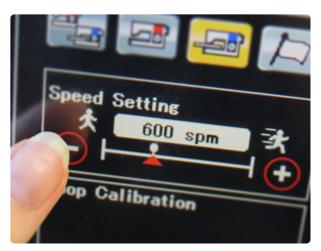
When you're working with any delicate thread, slowing down the embroidery speed can help prevent thread breaks.
