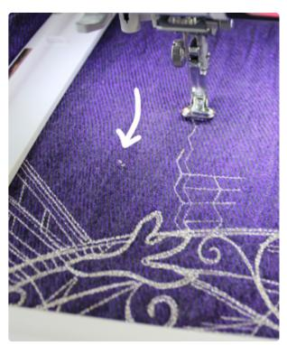
Once your fabric is under the machine, start your wing design stitching. Now, the first thing that will stitch is two alignment dots.
