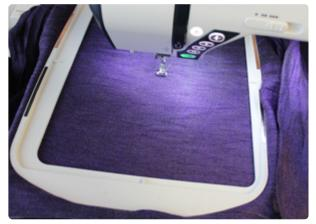
We're going to start in the middle and work our way out. Spray a piece of sheer mesh cutaway stabilizer with temporary spray adhesive, smooth it onto the back of your fabric, hoop them up together where you want your hawk body to stitch, and load up the hawk body design on your embroidery machine
