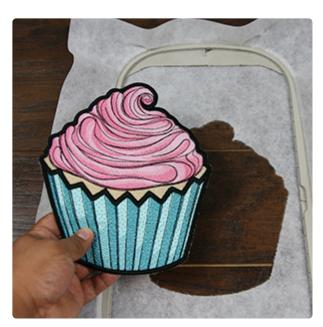
Place the bobbin into the machine so the bobbin matches the top thread. Follow the color change sheet to embroider the rest of the color change steps.
