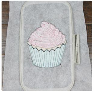
Remove the hoop from the machine, and turn it over so the back side of the embroidery is facing up. Lightly spray the back side of the back fabric piece with temporary adhesive and place the fabric piece inside the dieline.
