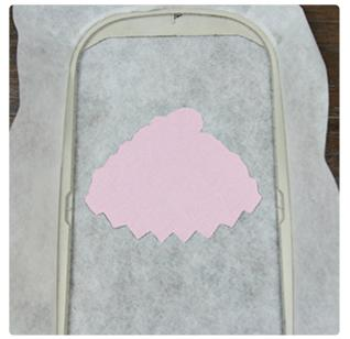
After the dieline has sewn, remove the hoop from the machine, but do not unhoop the stabilizer. Lightly spray the back side of the first fabric piece with temporary adhesive and place the fabric piece inside of the dieline.
