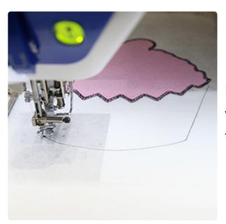
Return the hoop to the machine. A tackdown will stitch and hold the fabric piece in place for the remainder of the design.
