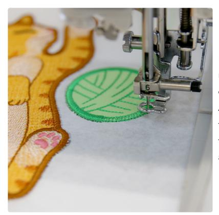
Load the matching bobbin into the machine, attach the hoop, and continue to embroider the design. A tackdown will sew first to hold the back piece in place. Then, a final border will sew around the accent bookmark shape.
