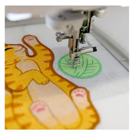
Then, place the hoop back onto the machine and embroider the tackdown for the accent, front fabric piece. The tackdown will hold the fabric piece in place for the remainder of the design.
