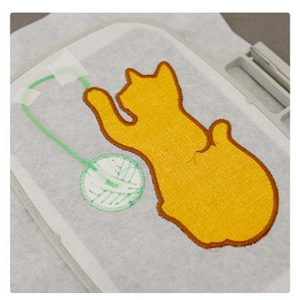
Remove the hoop from the machine but do not unhoop the stabilizer. Flip the hoop over, so the back of the hoop is facing up. Position the string, so the other end is slightly overlapping the fabric and embroider area of the accent piece. Then, tape it into place.
