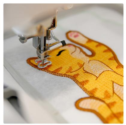
Load the matching bobbin into the machine, attach the hoop, and continue to embroider the design. A tackdown will sew first to hold the back piece in place. Then a final border will sew around the main bookmark shape.
