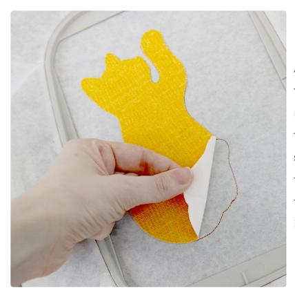
After the dieline has sewn, remove the hoop from the machine but do not unhoop the stabilizer. Spray the stabilizer side of the main shape's front fabric piece with temporary adhesive. Smooth the fabric piece onto the stabilizer inside of the sewn dieline.
