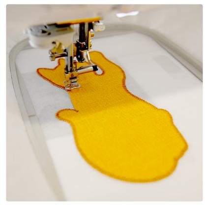
Then, place the hoop back onto the machine and embroider the tackdown for the main, front fabric piece. The tackdown will hold the fabric piece in place for the remainder of the design.
