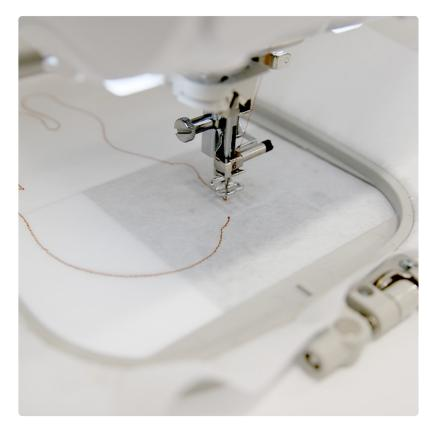
Attach the hoop onto the machine and load the embroidery file (not the dieline files). Use a 75/11 sharp sewing needle instead of an embroidery needle. The sharp sewing needle has a finer point and will make smaller perforations in the stabilizer.
