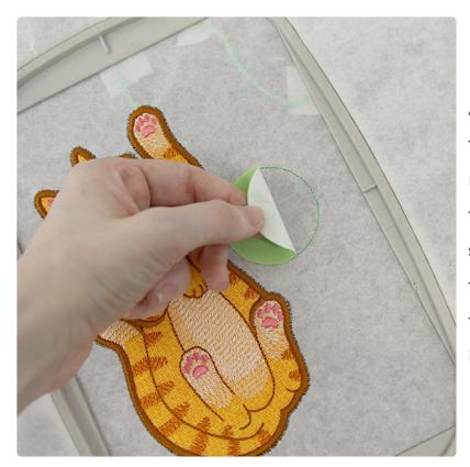
After the dieline has sewn, remove the hoop from the machine but do not unhoop the stabilizer. Spray the stabilizer side of the accent shape's front fabric piece with temporary adhesive. Smooth the fabric piece onto the stabilizer inside of the sewn dieline.
