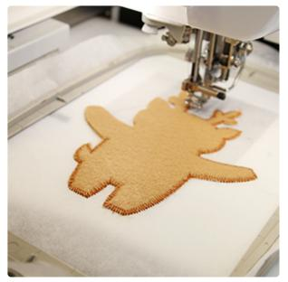
Attach the hoop back onto the machine and continue embroidering the design. The next step will tack down the fabric.
