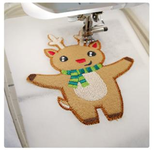
Attach the hoop in the machine and continue embroidering the design. A tackdown stitch will sew next, binding the layers together. Follow the final color changes.
