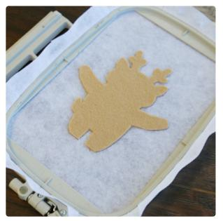
Remove the hoop from the machine, but do not unhoop the stabilizer. Spray the back side of the front felt piece with temporary spray adhesive, and place the fabric right inside the dieline.
