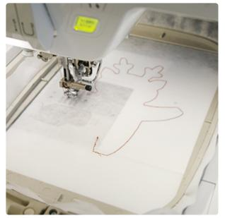
Attach the hoop to the embroidery machine and load the full embroidery design file into the machine. The first thing to stitch is a dieline that shows were to place the front felt piece.
