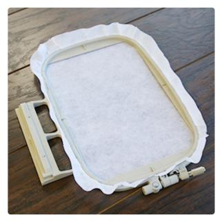
Once all of your pieces have been cut, hoop a piece of tearaway stabilizer taut. Use a size 11 or 75/11 sharp sewing needle rather than an embroidery needle (a sharp sewing needle has a smaller, finer point than an embroidery needle, so that it will make smaller perforations in the stabilizer).
