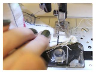
Pinch the four corners of your bag flat, about 1/2 inch up, and sew a seam at each corner. This will give it a bit of a "box" shape instead of just a flat pouch. Trim the excess off the corners.
