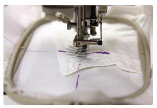
Once hoop is in position, make sure to align the needle with the center point of the design before embroidering.
