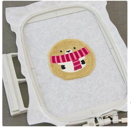
Once all the inner details are done embroidering, remove the hoop from the machine, but do not unhoop the stabilizer. First carefully remove as much of the watersoluble stabilizer as you can. It is usually easier to remove now but can be left until later if preferred. For Sulky Solvy, it is quite easy to just rip it off the design as it is perforated.
