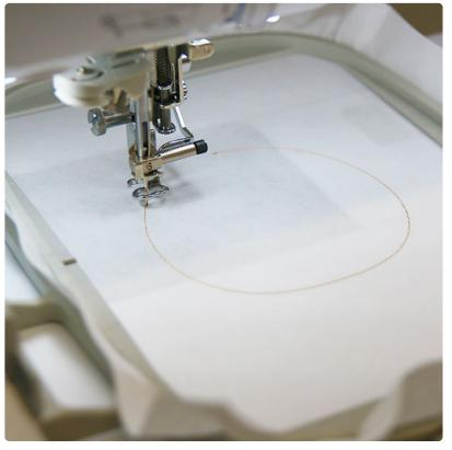
Attach the hoop onto the machine and load the embroidery file (not the dieline files). Use a 75/11 sharp sewing needle instead of an embroidery needle. The sharp sewing needle has a finer point, and it will make smaller perforations in the stabilizer. Embroider the design. The first thing to embroider will be the dieline (or outline stitch) for the front fabric piece. This marks the area on the stabilizer where the fabric piece will be placed.
