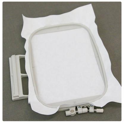
Hoop a piece of tear-away stabilizer firmly. Make sure it is nice and tight with no wrinkles.
