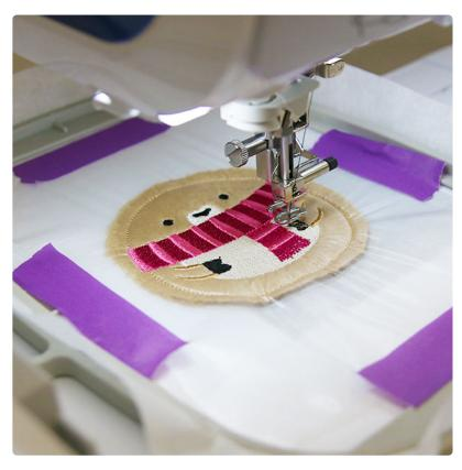
Then embroider the inner details of the design onto the front piece.
