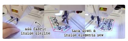
Lightly spray the back of your tag piece, and carefully place it inside the dieline. Once you set your machine to sewing again, it will stitch a tack down, holding your fabric in place. After that, all the inside elements will stitch out.
