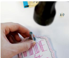
Place the backing piece behind it, and use your grommet tool to hammer the two pieces together. Be sure to do this on a hard sturdy surface! Though you see this on my desk, it's probably much better to do this on a hard floor.
