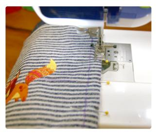
To stop the seam from unraveling, I'm going to create a French seam.
