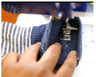
Then, flip the cuff right side out, and fold all the seam allowance toward the opening. The raw edge should be completely covered. Sew inside the cuff, close to the edge as shown, making sure the raw edge is completely enclosed in the seam.
