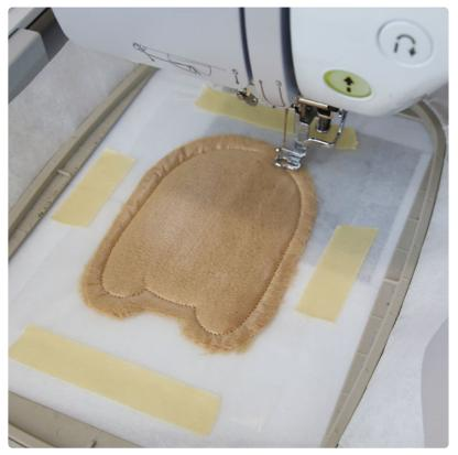
Place the hoop back onto the machine and embroider the tackdown for the front fabric piece.
