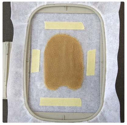
To prevent the embroidery from sinking into the fluffy fabric, cut out a piece of light weight watersoluble stabilizer that is larger than the design (we used Sulky Ultra Solvy). Lay it over the front fabric piece and tape the edges down onto the hoop or stabilizer around the design.
