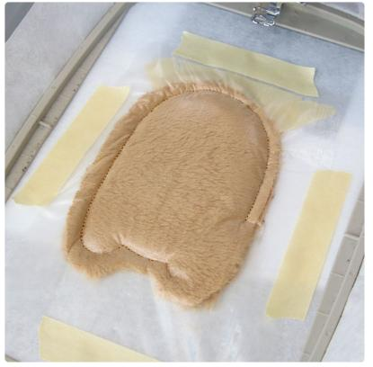
Place the hoop back onto the machine and embroider the back piece tackdown. This will adhere the front and back pieces together. It will also leave a small opening along the edge for turning.
