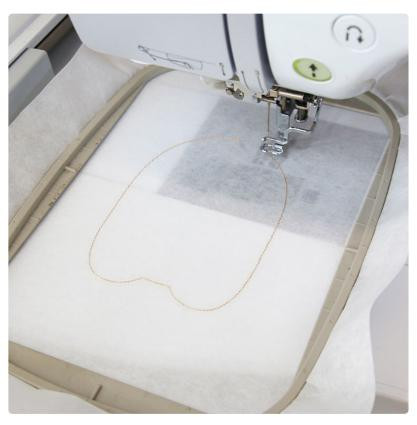
Attach the hoop onto the machine and load the embroidery file (not the dieline files). Use a 75/11 sharp sewing needle instead of an embroidery needle. The sharp sewing needle has a finer point, and it will make smaller perforations in the stabilizer.
