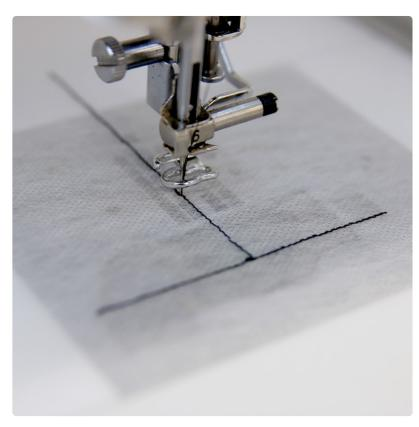
Attach the hoop onto the machine, and load the embroidery file (not the dieline file). Begin to embroider the design. For best results, use a size 11 or 75/11 sharp sewing needle. This needle has a smaller point, and it will make smaller perforations in the stabilizer which helps prevent shifting and tearing.
