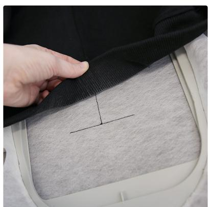
After sewing the "edge and seam placement lines", remove the hoop from the machine, but do not unhoop the stabilizer. Spray the wrong side of your garment with temporary adhesive, and smooth it into place on top of the placement lines.
