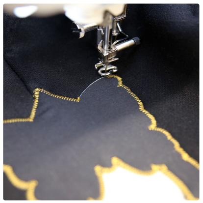
Then place the hoop back onto the machine, and embroider the tackdown for the first applique piece that was just placed. A tackdown holds the fabric piece in place for the remainder of the design.
