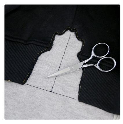
Remove the hoop from the machine, but do not unhoop the stabilizer. With a scissors, carefully cut along the inner edge of the sewn "cutline" to make the opening for the split seam. Make sure to leave no more than a 1/8in along the inner edge.
