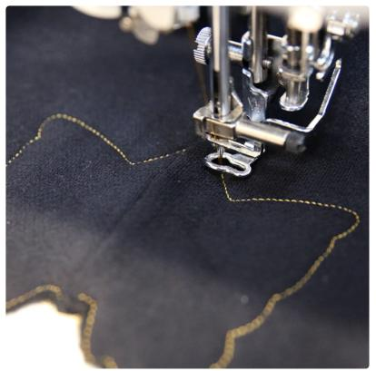
After cutting, place the hoop back onto the machine, and continue to embroider the design until the step with "dieline" in the text has sewn out. The dieline (or outline step) marks the area where the applique piece will be placed. Some designs will have the dieline will sew right away, and other designs will have some details that sew before the dieline.
