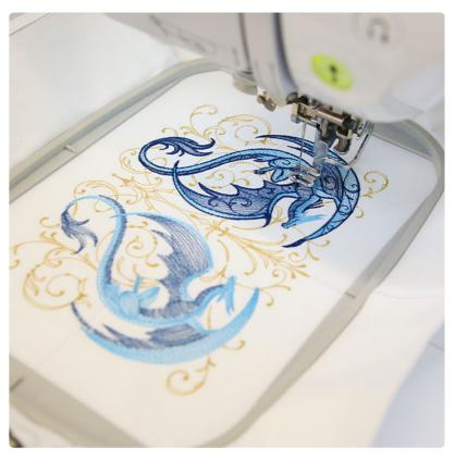
Load the embroidery file onto the machine and secure the hoop in place. Then move the needle directly over the marked center point on the fabric. Follow the color change sheet and embroider the design.
