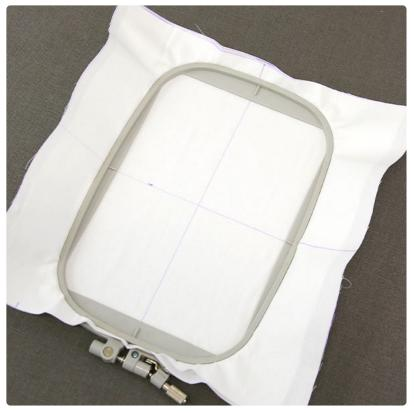
Then hoop the fabric and stabilizer together so that they are drum tight, lining up the drawn axis lines with the marks on the hoop.
