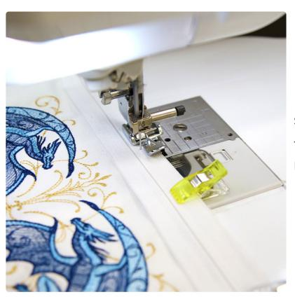
Stitch the fabric and zipper together using a zipper foot leaving about 1/4" seam allowance.
