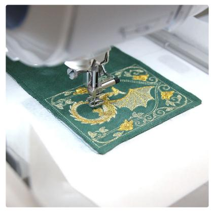
Attach the hoop back onto the machine and continue with the design. A running stitch tackdown will sew next. This holds the front fabric in place for the remainder of the design. Then follow the color change sheet to embroider all the inner details. Stop before sewing the "finishing seam step".
