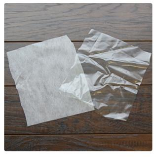
There are a couple of different kinds of heavy water-soluble stabilizer. One is clear and plastic, and that brand is Sulky Ultra Solvy. The other is soft and fibrous, called Vilene. Both will work very well. Vilene is used in this demonstration.
