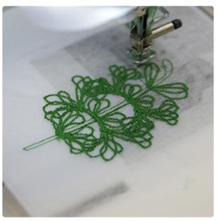
Attach the hoop to the machine and load the embroidery file. Follow the color change sheet, and embroider the first color of the design using a matching bobbin.
