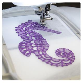
Attach the hoop to the machine and load file "a".
