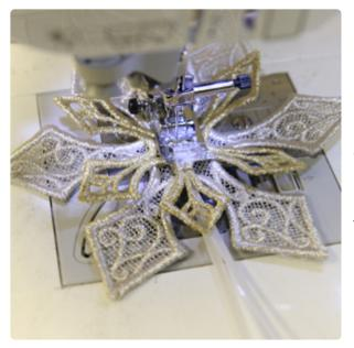
Place the center of lace piece "b" over the center of lace piece "a" and stitch the two pieces together. Make sure you thread matches the embroidery design.
