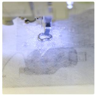
Attach the hoop to the machine and begin sewing the embroidery design. Repeat the previous steps when sewing parts "b" and "c" of the design.
