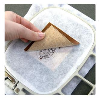
After the inner detail and "hole punch guide" have sewn, remove the hoop from the machine. Do not unhoop the stabilizer. Turn the hoop over so the back side is facing up. Spray the back fabric piece with temporary spray adhesive. Then, smooth the back fabric piece over the shape on the back side.
