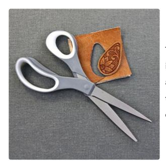
Then, using scissors, carefully cut along the inner edge of the "cut line" from earlier. Cutting along the inside of the cut line will remove those stitches from the leather piece, leaving a clean and smooth edge.
