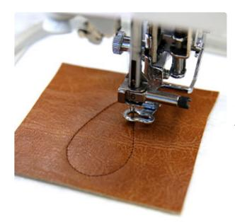
Next, place the hoop back onto the machine and embroider the "front piece tackdown." A tackdown holds the fabric piece in place for the remainder of the design.
