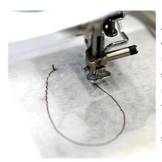
Attach the hoop to the machine and load embroidery file 'A.' Use a 75/11 sharp sewing needle instead of an embroidery needle. The sharp sewing needle has a finer point and it will make smaller perforations in the stabilizer. The first thing to embroider will be a "fabric dieline" (or outline stitch). This marks the area on the stabilizer where the fabric piece will be placed.
