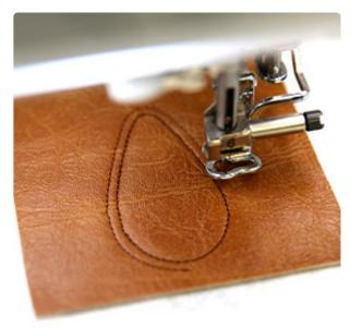
The next step to embroider will be the "cut line." This marks the area on the leather where the finished design will later be cut out.
