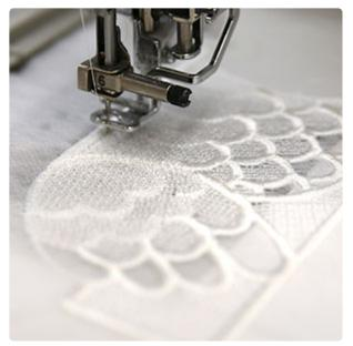
Attach the hoop to the machine and load file
