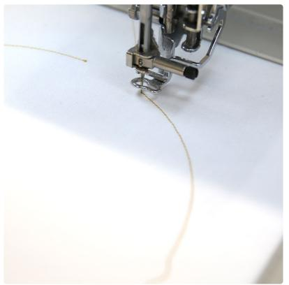
Attach the hoop to the machine and load the second part of the design or file "B". The first thing to stitch out will be the dieline. Unlike the previous dieline, this one will be used for placement.
