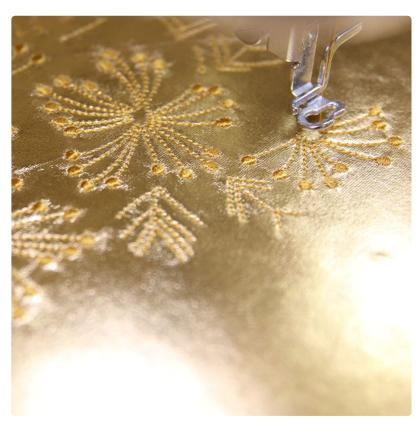
Attach the hoop onto the machine and load the first hooping or embroidery file - "Piece A". Use a size 11 or 75/11 sharp sewing needle rather than an embroidery needle. A sharp sewing needle has a smaller, finer point than an embroidery needle. This will make smaller perforations in the stabilizer, providing more support.
