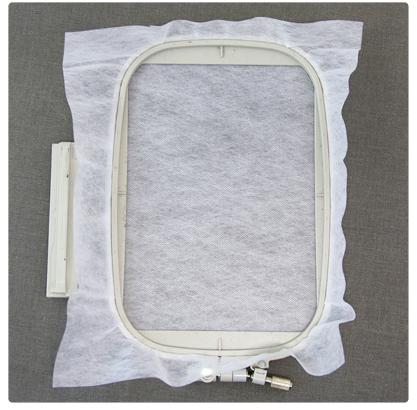
Hoop the water-soluble stabilizer together firmly. Make sure it is nice and tight with no wrinkles.
