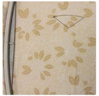
After the design file has been loaded onto the embroidery machine, start stitching. The machine will stop after the first step stitches out. This will be the dieline, for applique placement.
