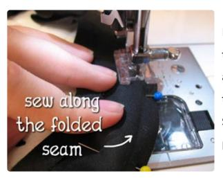
Now we're going to sew our first seam around the edge. Stick it under the sewing machine, and line your needle up so it's going to follow that indented seam left behind by the fold. Stitch carefully along that line, removing the pins as you go, until you're all the way around.
