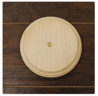
Use a drill with a 3/8" drill bit to create a 1/4" to 1/2" deep hole (to place the wooden dowel in), and clear the sawdust.
