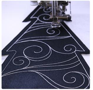
Follow your color change sheet and continue to stitch the remaining details. Watch for the step that says "back piece tack down". When you reach this step, remove the hoop from the machine once again, but do not unhoop the stabilizer.
