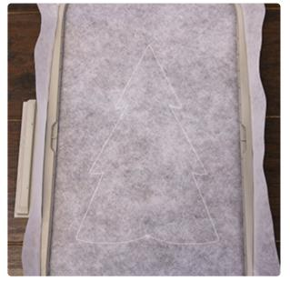
Once all of your pieces have been cut, hoop a piece of tearaway stabilizer taut. Use a size 11 or 75/11 sharp sewing needle rather than an embroidery needle (a sharp sewing needle has a smaller, finer point than an embroidery needle, so that it will make smaller perforations in the stabilizer).
