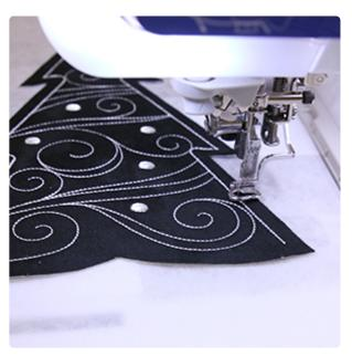
Attach the hoop to the machine and continue embroidering the design. A tackdown stitch will sew next, binding the layers together and leaving an opening at the bottom of the design.
