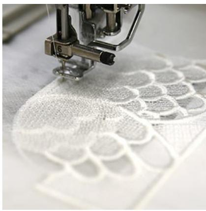
Attach the hoop to the machine and load file "a." Follow the color change sheet and embroider all of the design using a matching bobbin.
